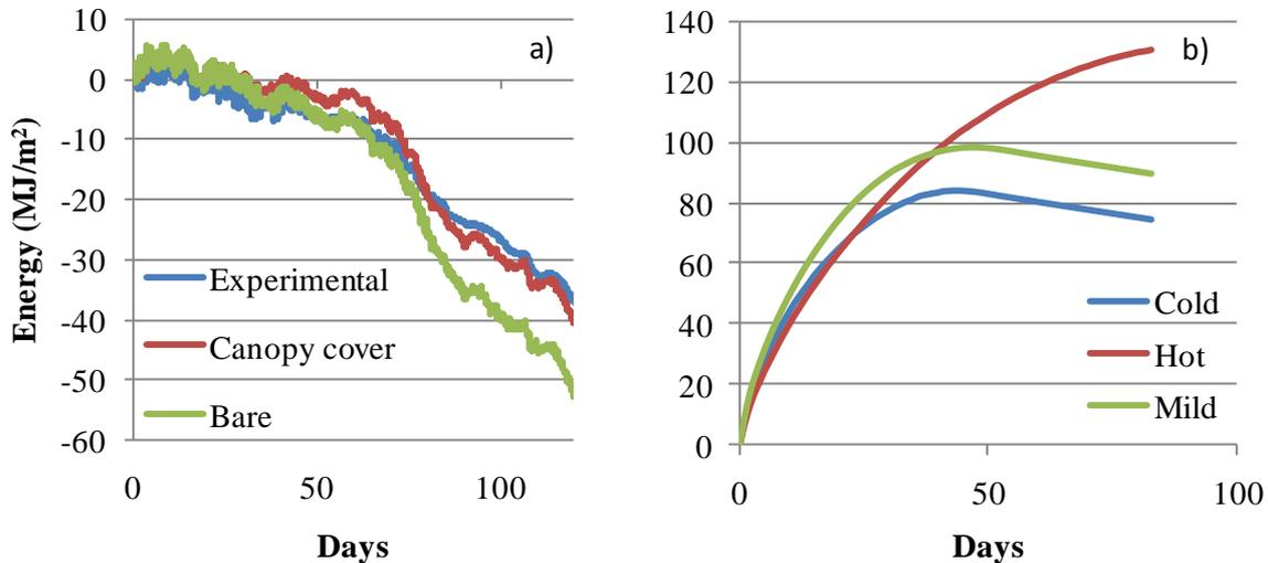
**Figure 3 - a) Effect of theoretical formulation of heat balance at the soil surface on the amount of thermal energy stored in the far field ground. b) Influence of weather conditions on amount of estimated thermal energy collected by the system. Day 0 corresponds to 23/08/05.**
