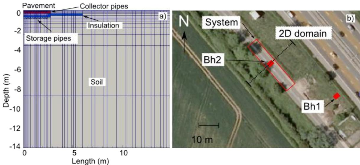
**Figure 1 - a) Half of domain used in this work showing position of main elements. b) Position of experimental system and boreholes used in this work and approximate position of 2d domain.**
