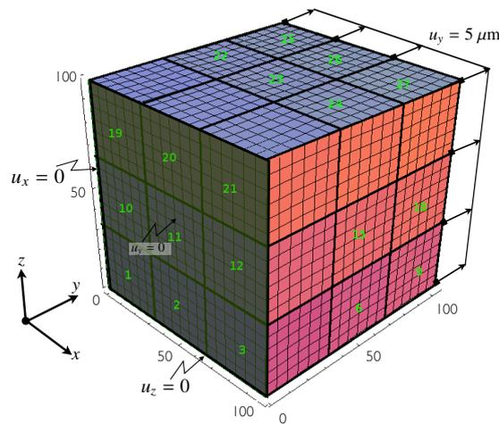
Figure 1: Discretization of the polycrystal composed of 27 grains.
