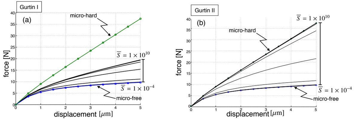
Figure 2: Applied displacement versus the  $y$ -component of resultant force on the right boundary for various grain-boundary models. The results of the Gurtin I model are shown in (a), and the Gurtin II model in (b).
