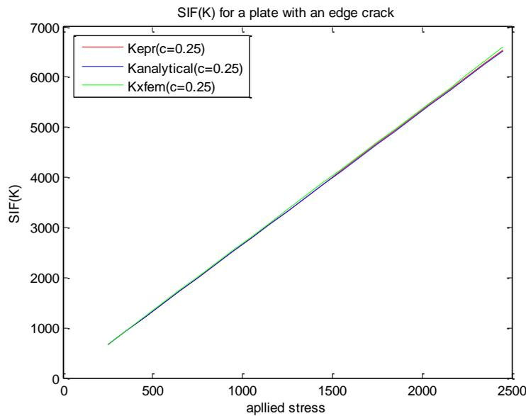
Figure 3. Stress intensity factor (K) vs applied stress
