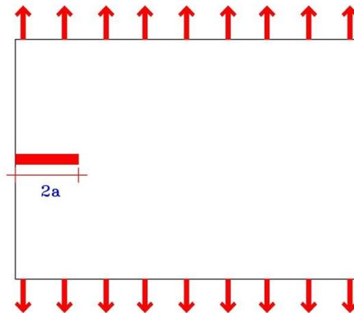
Figure 2. Tensile Plate with an edge crack.
