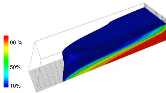
Figure 3: 3D salinity map (%) of hypothetical example prior to recharge process
