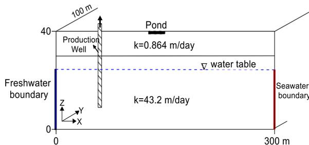
Figure 1: Geometry and boundary conditions of the hypothetical model
