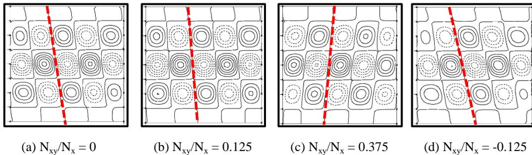
Fig. 5. VICON mode shapes of stiffened panel ST 2-1 for four different interaction ratios.
