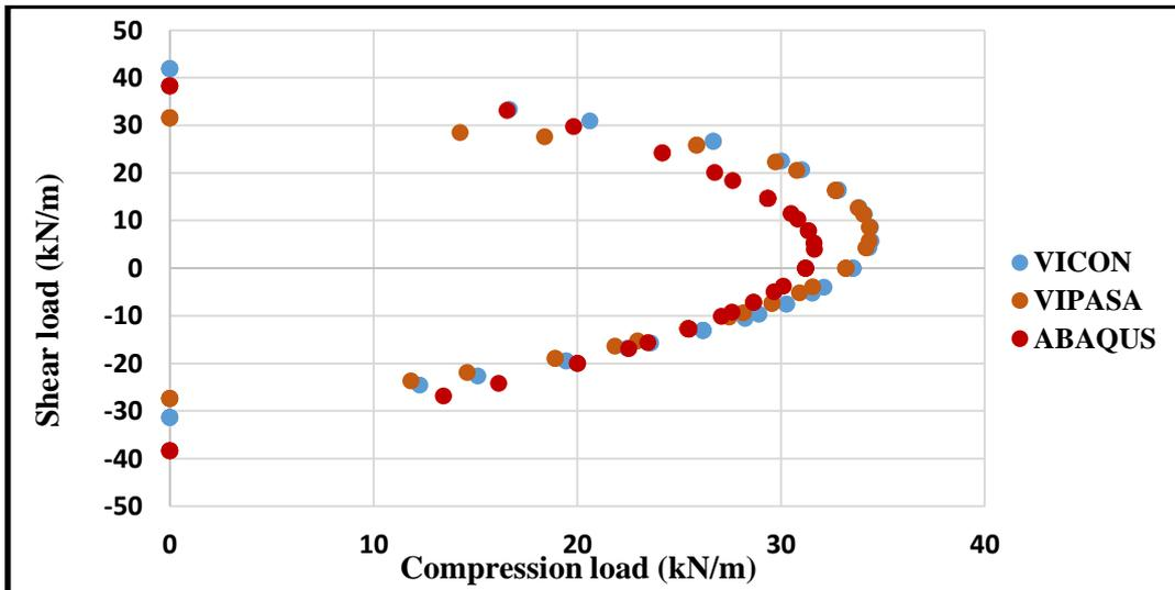
Fig. 2. Interaction curve for stiffened panel ST 1-1.
