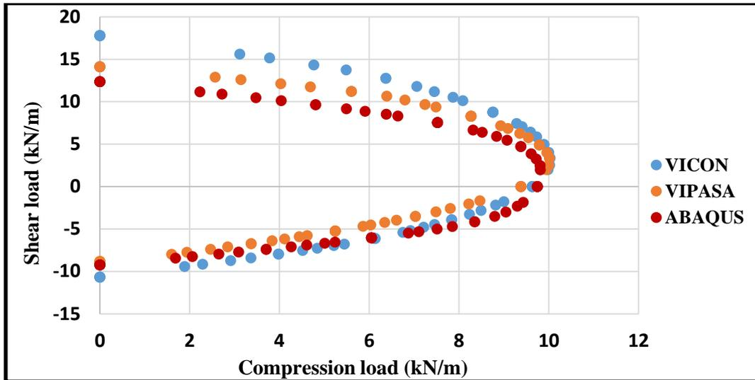
Fig. 1. Interaction curve for flat plate FL 2-3.
