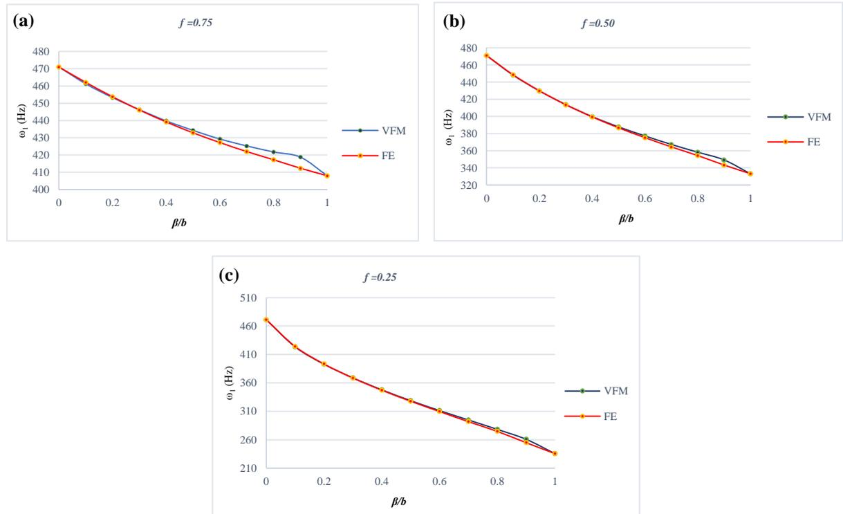
Figure 2: Plots of lowest natural frequency ( $\omega_1$ ) against width  $\beta$  of centrally located through-the-length damage, for different values of stiffness reduction factor  $f$ . (a)  $f=0.75$ , (b)  $f=0.50$ , (c)  $f=0.25$ .
