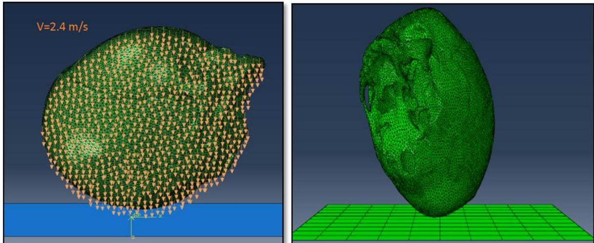
Figure 2: Illustration of (a) the boundary value problem of an occipital impact to a 10 day old infant head (with skull, sutures, and brain), and (b) Finite element (FE) simulation of the same.
