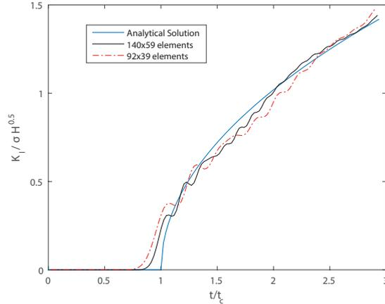
Figure 3: Normalized mode I stress intensity factor against normalized time for a stationary semi-infinite crack. The analytical solution is plotted as well as the computational solution considering two different discretizations: 92 by 39 and 140 by 59 elements .
