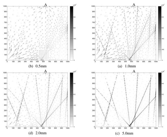
Figure 2: Velocity vectors for various fracture apertures
