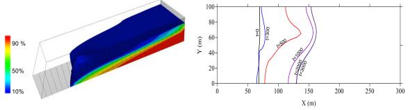
Figure 3: 3D salinity map (%) of hypothetical example prior to recharge process
