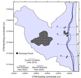
Figure 6: Inland progress of 50% iso-concentration lines across the base of Wadi Ham aquifer
