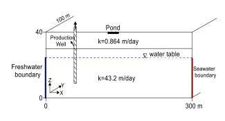
Figure 1: Geometry and boundary conditions of the hypothetical model
