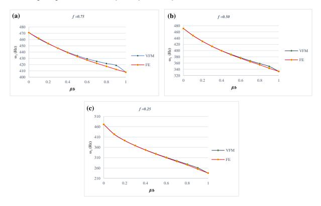
Figure 2: Plots of lowest natural frequency ( $\omega_1$ ) against width  $\beta$  of centrally located through-the-length damage, for different values of stiffness reduction factor *f*. (a) *f* =0.75, (b) *f* =0.50, (c) *f* =0.25.
