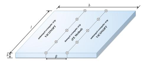
Figure 1: VICONOPT and FE method modelling damaged plate
