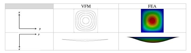
Figure 3: VFM and ABAQUS plots of lowest natural frequency mode for plate with through-the-length damage of  $\beta/b=0.2$
