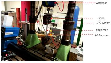
Figure 2. Experimental fatigue test setup
