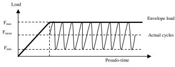
Figure 6. Schematic of fatigue modelling envelope load
