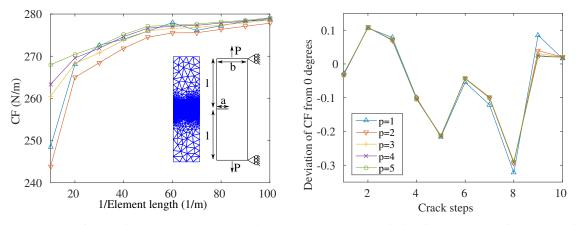
(a) CF value for varying element length and local p- (b) CF angle deviation from 0 degrees for a developing adaptivity at crack tip.
